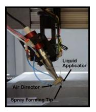
Fig. 1: Nozzle-less Ultrasonic Spray Head Assembly
