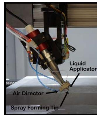
Fig. 1: Nozzle-less Ultrasonic Spray Head Assembly
