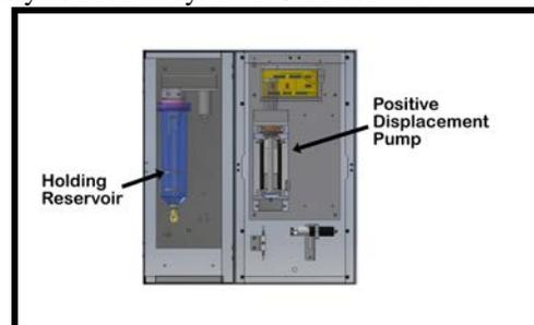
Fig. 2: Liquid Delivery System
